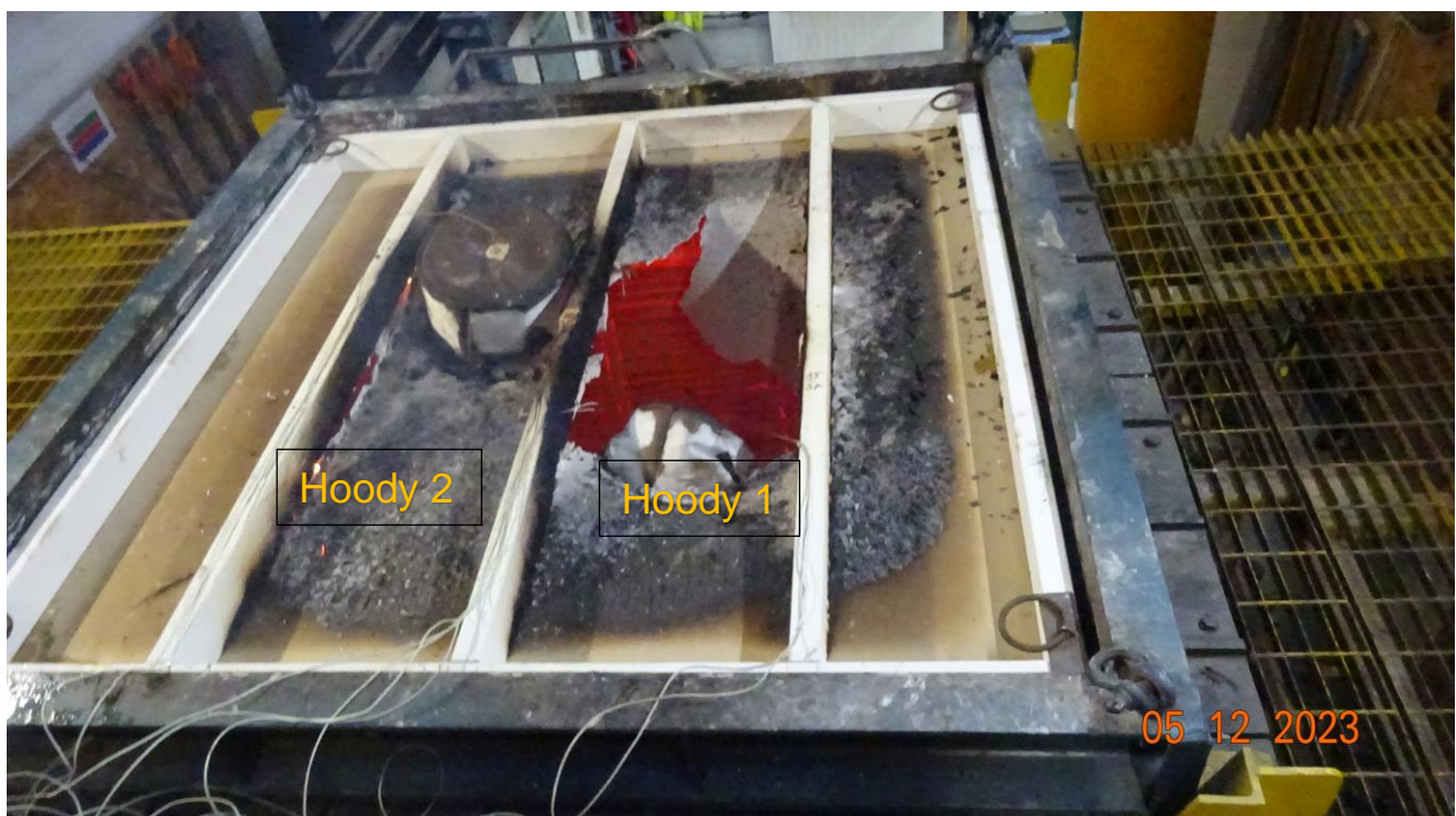
Image of unexposed face of specimen at 107 minutes (end of test)
